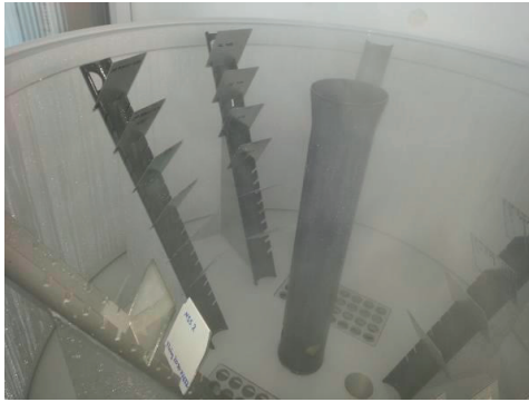
Fig. 3: Salt spray chamber for NSS or CASS tests.
