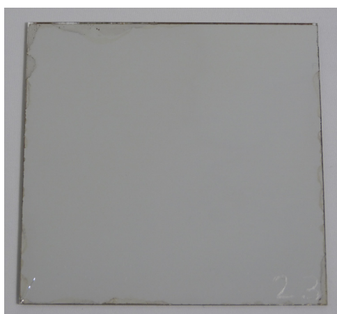
Fig. 9. Picture of sample 2, after the humidity test.
