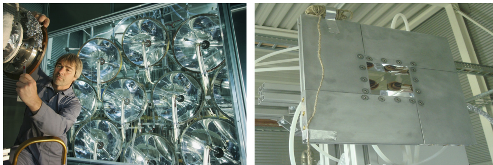
Fig. 6. High flux simulator (left) and frontal view of the OMX (right) at PSI.
