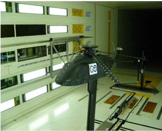
Figure 1: The GOAHEAD configuration inside the DNW-LLF wind tunnel
