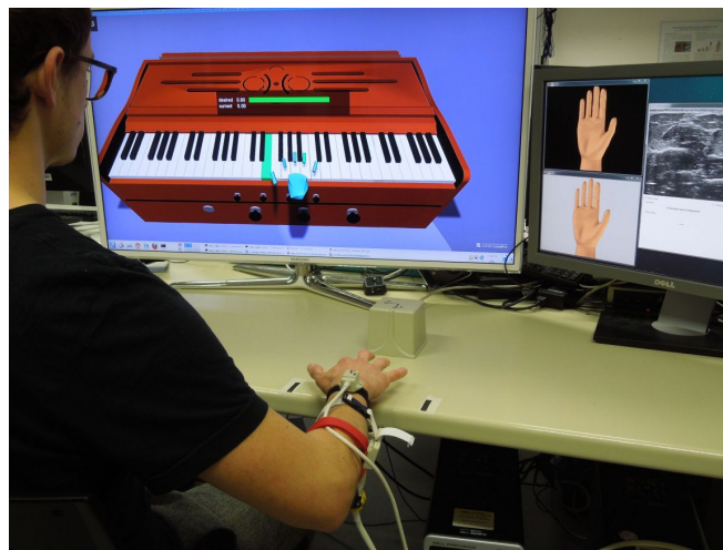
Fig. 1. The virtual-harmonium setup has three main components: an ultrasound machine capturing images of the forearm, a magnetic tracker to detect the hand movement and a realistic virtual reality environment.
