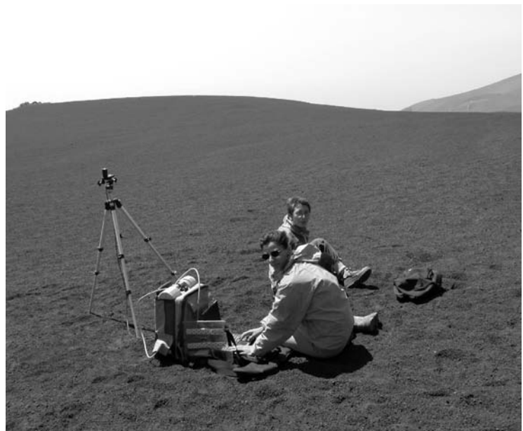
Figure 5.30 Measurements configuration .The remote sensing receptor was mounted at the cable fore optic over a tripod at 145 cm ground altitude.
