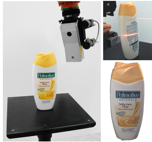
Fig. 2. Autonomous object modeling of a shower gel. Left : Laser striper and stereo camera are attached to the flange of an industrial robot. The unknown object is placed on a pedestal. Top right : Image from bottom mono camera view. Bottom right : Textured 3D Model.
