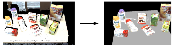
Fig. 4. Left: A scene acquired by the SGM stereo algorithm; Right: The estimated supporting plane and clustered scene.
