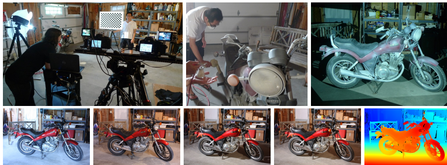
Fig. 4. Top: Portable stereo rig with 2 DSLRs and 2 consumer cameras, and painting of glossy scene. Bottom: Ambient views under different lighting conditions and disparities.
