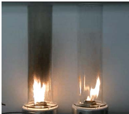
Fig. 5: Burning of a GtL (right) and of Jet A-1 (left) showing clearly the lower sooting propensity of a GtL fuel [32]
