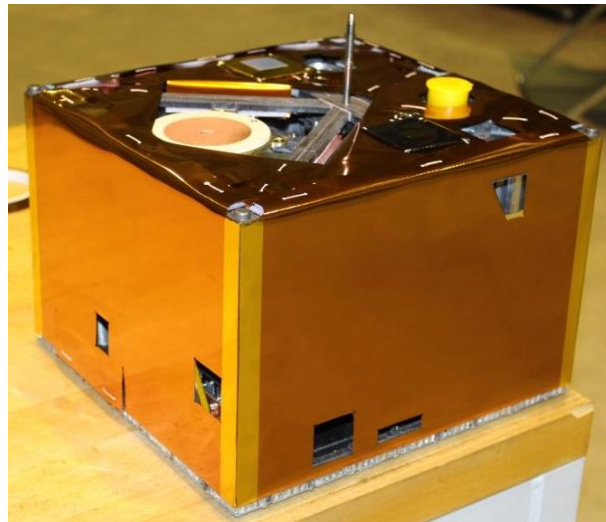
Fig. 6: MASCOT (bottom view) with separation mechanism and windows for GNC sensors
