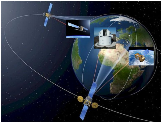
Fig. 1. Artist's impression of two EDRS satellites in GEO servicing Sentinel 1a and 2a in LEO as well as ESA's OGS
