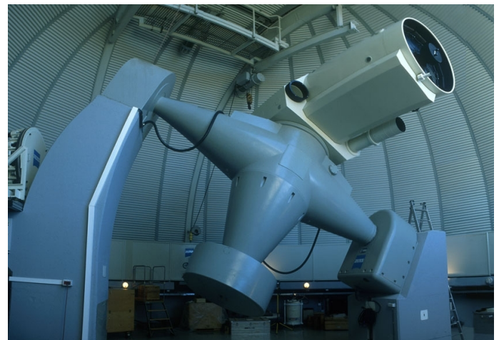
Fig. 6. The English mount of the 1 meter Zeiss telescope
