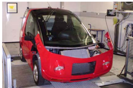
Fig. 9: Test platform to install a drive motor with integrated air conditioning compressor
