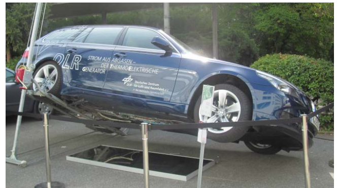
Fig.16: Test platform with thermoelectric generator in the exhaust system based on a BMW 5series
