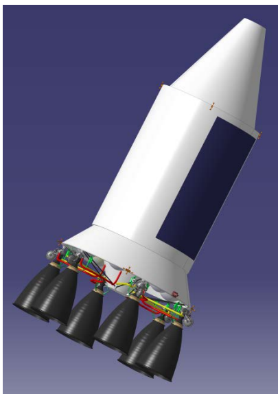
Figure 9: Side view of the high-thrust stage (body mounted solar panel in blue)
