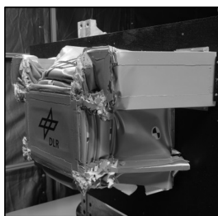
Fig. 19: Front structure of the LUV before and after crash test
