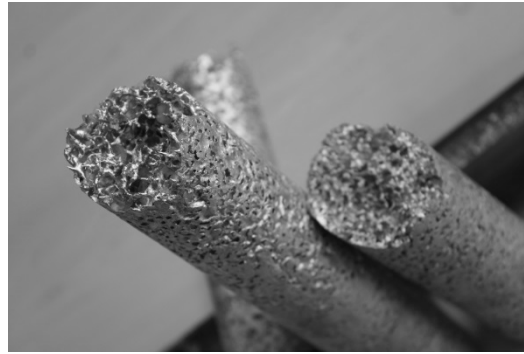
Fig 15: Aerofims –Metal-Aerogel Composites made by suction casting.
