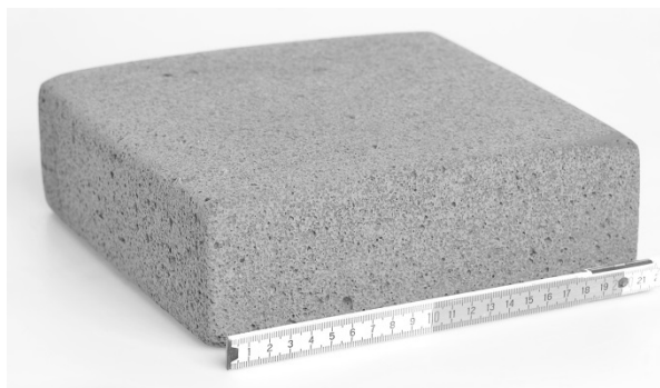
Fig. 13 shows an example of a polymeric aerogels in which silica aerogel particles are embedded yielding a light weight material with superisolating properties and good sound absorption.
