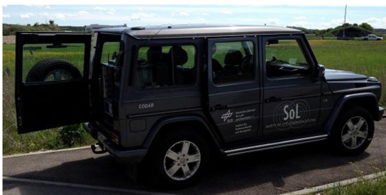
Figure 5. DLR integrated test vehicle (the On-Board Unit is installed in the trunk, and the two antennas are located on the roof of the vehicle).
