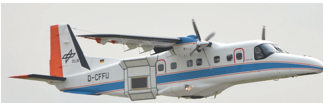
Figure 1. The F-SAR sensor installed on a Do-228-212 aircraft with the Antenna Carrier for the X, C, S and L-band antennas towards the aft
