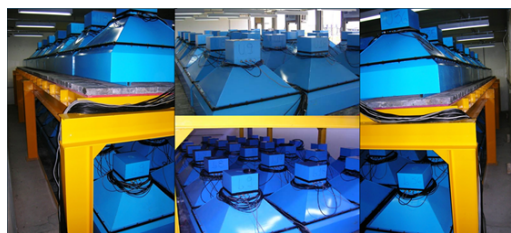
Fig. 2: Multidirectional Muons Detector (MMD) of Cooperation Japan-USA-Brazil, installed in the Southern Space Observatory, in São Martinho da Serra, Southern Brazil.
