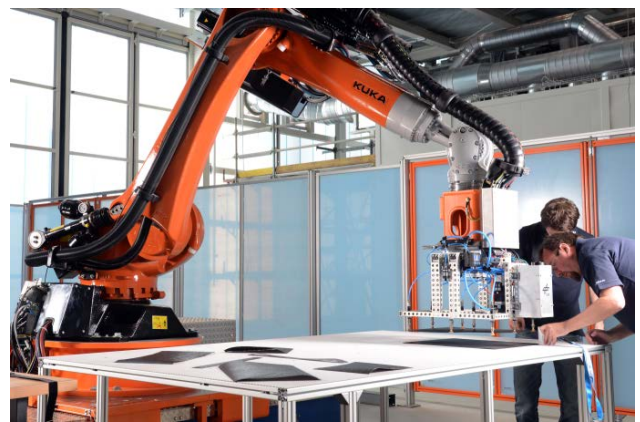
Fig. 17: Robotic end effector with automated cut piece detection for gripping, lay-down and fixation of CFRTP fabrics.
