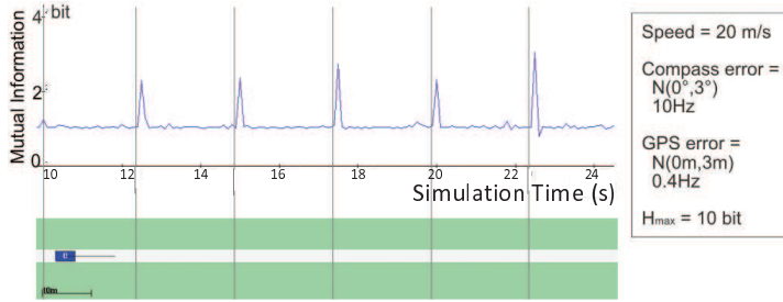
Figure 11: Mutual information on a straight road with GNSS position fixes every 2.5 s.
