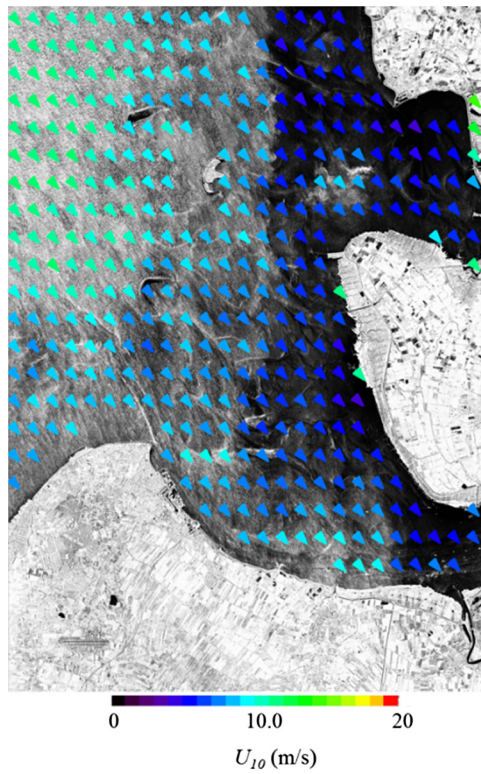
Fig. 22 Wind field derived using the XMOD algorithm for the TS-X acquisition taken on November 21, 2008, at 17:01 UTC over the Elbe estuary.
