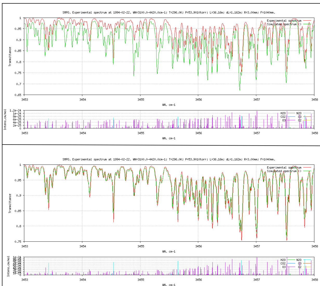
Figure 5. Example of an improvement of the Q branch for the \nu_1 + 2\nu_2 + \nu_3 ozone band. The top panel is a comparison of the observed spectrum (in red) with calculations using HITRAN2008 data (in green); the bottom panel is a calculation with new data from S&MPO (including a few impurity lines marked in blue in the stick diagram).
