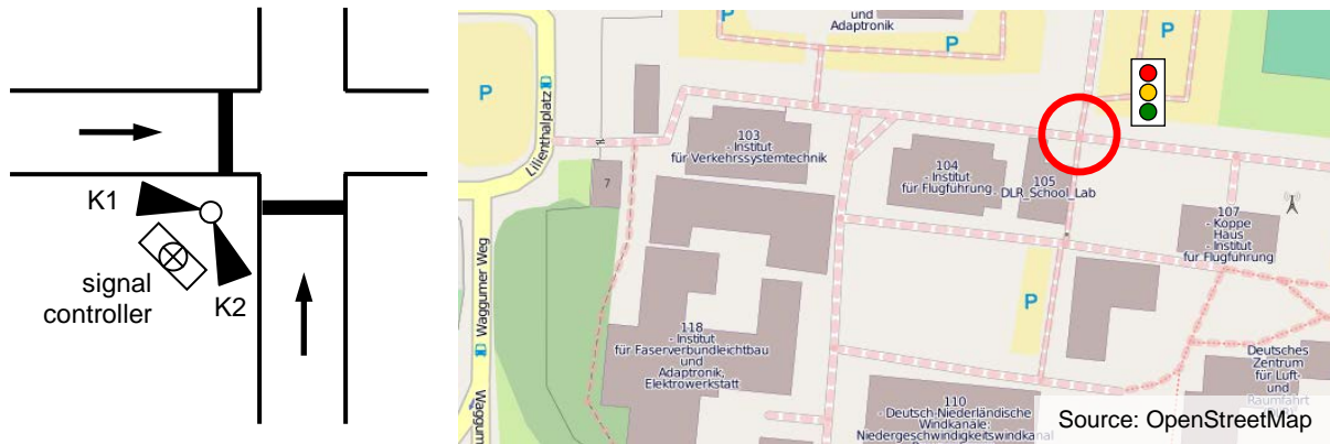
Figure 4: The test site is a simple intersection consisting of two crossing one-way streets, each signalized by a separate signal group (left). The intersection is located at the non-public property of the DLR in Braunschweig (right).
