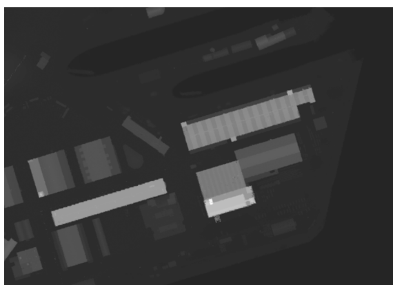
Fig. 17. A DSM model created from the LiDAR data provides the basis for the geometry model.
