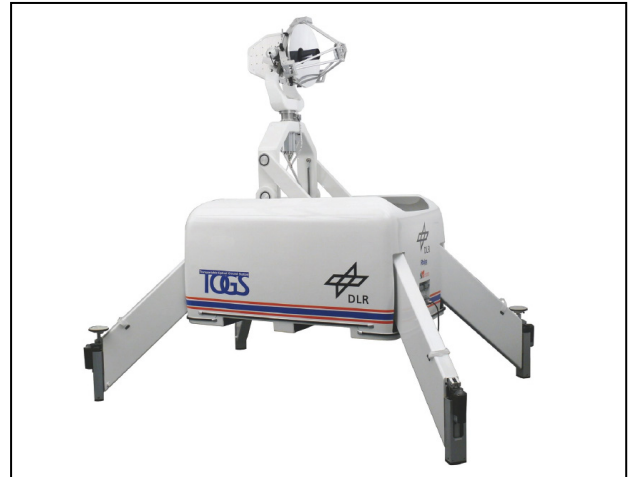
Figure 4. Transportable Optical Ground Station (TOGS): 60cm aluminium mirror, whole mount foldable into box for air-freight
