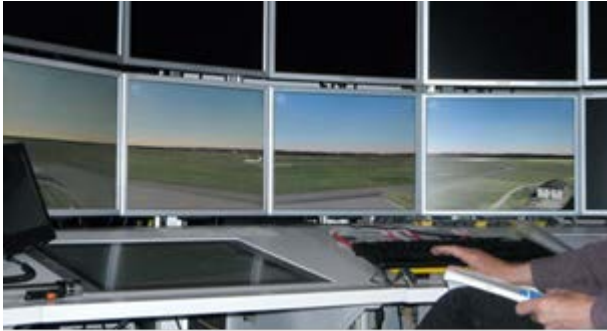
Figure 29: Participant at a simulation console judging the outcome of a landing aircraft just after touchdown. Approach on the rightmost monitor, touchdown is on the left side of second monitor from the right.
