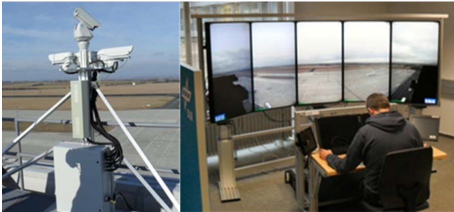
Figure 2: Left: RTO sensor system with five HD-format panorama cameras and pan-tilt zoom (PTZ) camera on top, mounted on roof platform of Erfurt-tower (height 41 m). (see contribution of Schmidt). Right: RTO videopanorama display system with five HD-format displays for 200° view. Setup at DLR RTC-Simulator facilities for live transmission from Erfurt airport (200 km, with 50 Mbit/s)
