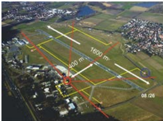
Figure 1: Braunschweig Airport with main runway in east–west direction. Red lines indicate camera segments of initial 180° high resolution (UXGA) video panorama system, operating 2004-2012; red circle: camera location; yellow lines: fiber-optic high speed data network, thick line indicating 600 m Gbit link for video transmission.
