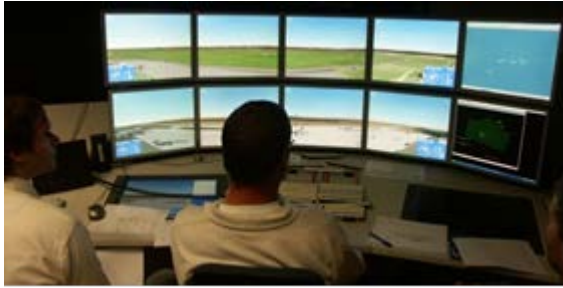
Figure 25: Remote Tower simulation with two-airport control by two operators (executive and coordinator)
