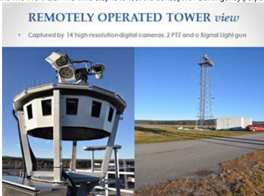
Figure 31: LFV/Saab Remote Tower sensor system (2012)
