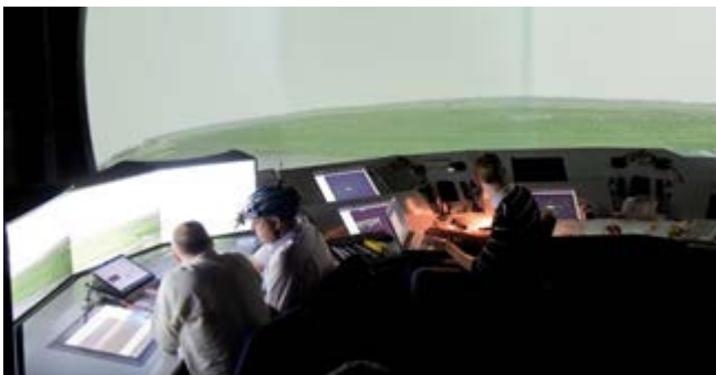
Figure 24: Remote Tower simulation setup (left console with two operators) within the Control Tower Simulator
