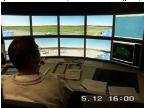
Figure 5: Dual airport control by single operator (see contribution of Möhlenbrink et al., section 11, [34][35][36][39][42])
