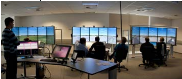
Figure 4: DLR Simulation Facility for Remote Tower Center Human-in-the-loop experiments (see contribution of A. Papenfuß, section 4)
