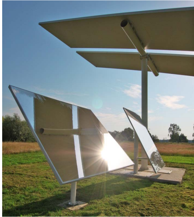
Fig. 5. Laminated mirror facets for heliostats
