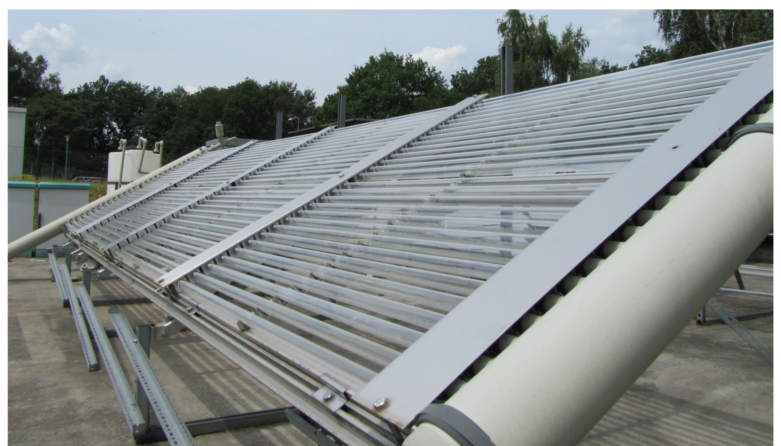
Fig. 2: Solar prototype reactor with non-concentrating tubular receiver modules at DLR, Cologne, Germany
