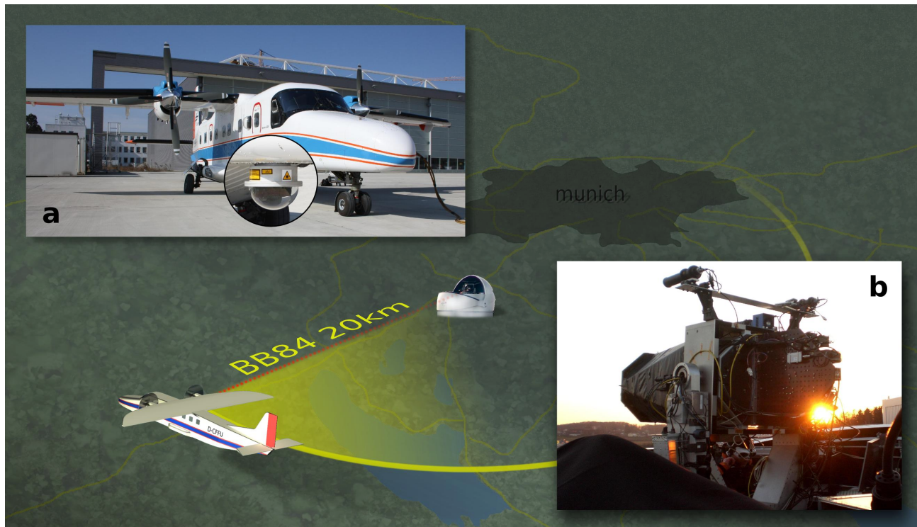
Figure 1. Experiment scenario: a The Do228 aircraft equipped with the flight terminal. The inset shows the optical dome underneath the fuselage housing the coarse pointing assembly (CPA). b , the optical ground station (OGS) of the German Aerospace Center's institute of communications and navigation. The normally open framework of the telescope was covered here to shield against stray light. All optics is mounted to the breadboard attached to the back of the main mirror.
