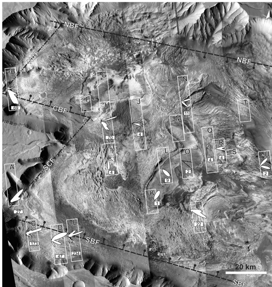
Figure 15. Histograms for the trends of fault traces recorded in each HiRISE image location. The number of data points, N , for each image is recorded to the bottom right of the histogram, and the size of each histogram has been scaled relative to the N value ( >20 = \text{large} , \leq 20 = \text{small} ).
