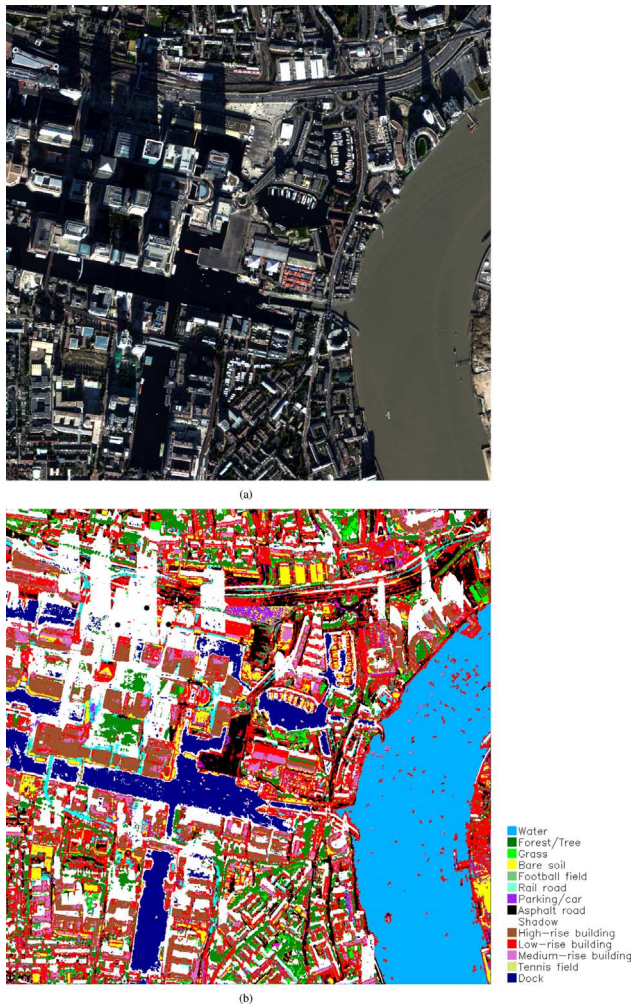
Fig. 16. London test area. Full size image employed for the FG fusion and classification. (a) visible range multispectral image (bands 5,3,2), (b) FG fusion and classification (WV-2+Texture (SAR and Optical)+DSM).
