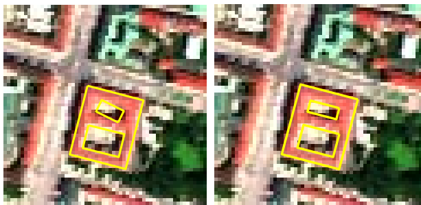
Figure 4: Result of building boundary approximation with sub-pixel accuracy (yellow lines). Outer and inner building boundaries are: independently adjusted (left), and adjusted with the condition that they have the same orientation (right).
