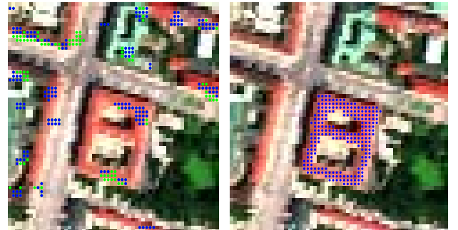
Figure 3: Left: The seed points selected from CartoSat DSM with removed vegetation and small regions (blue and green points) and remaining seed points after statistical refinement regarding spectral characteristics (blue points). Right: Result of region growing and merging of the central building (blue points).
