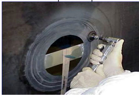
Fig. 3.7.1 Manual scarfing by angular grinding [5].
