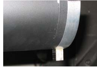
Figure 2. Pitot rake mounted on afterbody
