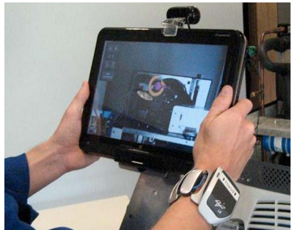
Figure 2: Mobile AR component including haptic bracelet
