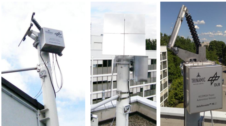
Figure 6: Test heliostat with dummy facets.
