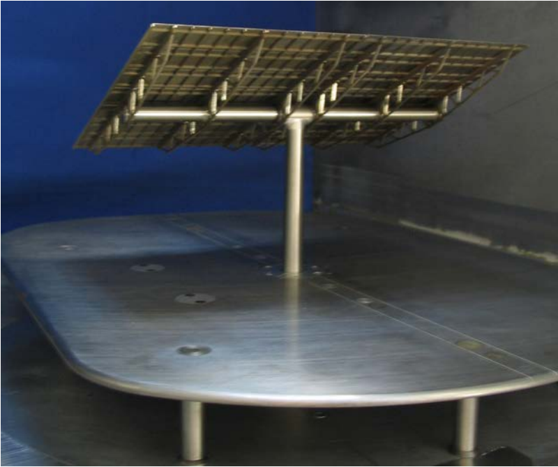
Figure 6: Heliostat model in HDG, scale 1:50
