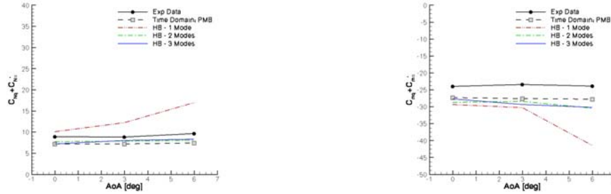
Figure 12. Normal force and pitching moment coefficient dynamic derivatives for V_\infty=56\text{m/s} , \alpha_A=4.5^\circ , frequency f=4.5\text{Hz} .
