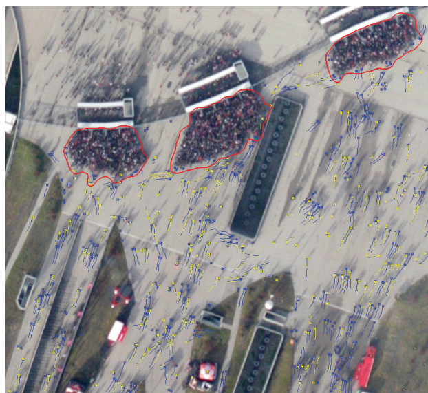
Figure 7: Results of the tracked people (yellow) and the reference data (blue), the tracks are pruned to the last six frames. The detected dense crowds are shown with red boundaries.
