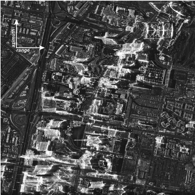
Fig. 1. Temporal multilook image of the spotlight TSX data set over the city of Las Vegas. The layover induced by the buildings is well recognizable.
