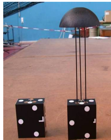
Figure 2. Overview on different experimental cargo bodies. The right body's CFRP rods have a length of 465 mm. A similar body with a rod length of 215 mm was also used in experiment and chosen for the validation of the numerical simulation.
