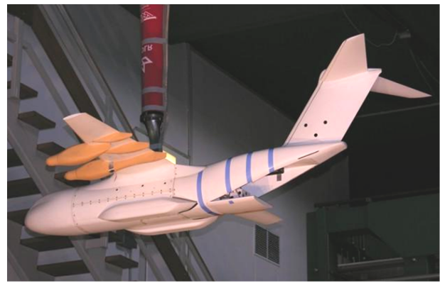
(b) Wind tunnel airdrop setup using a generic transport aircraft with lowered ramp.
