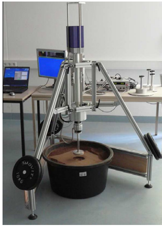
Fig. 2. Bevameter for soil characterization.
