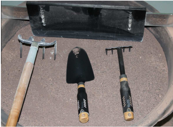
Fig. 4. Tools used for soil preparation method testing: levelling board (top), garden rake (left), hand shovel (middle) and little hand rake (right).
