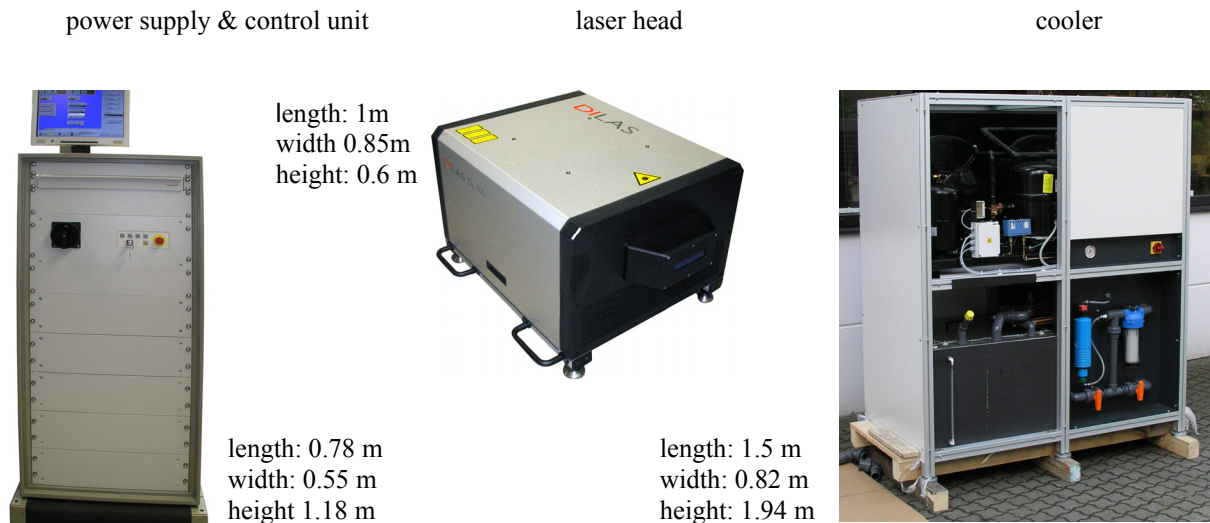
Figure 2: Components of the laser system: power supply & control unit (left), laser head (middle) and cooler (right).
