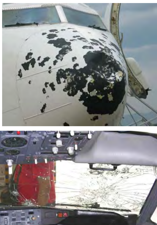
Figure 1: Nose and wind shield damage of two aircraft hit by hail stones during passage of thunderstorms. Left: Easy Jet Boeing 737 after take-off from Geneva, 15 August 2003. Right: WindJet A319 near Catania on Oct 1st 2009 (The Aviation Herald, Photo: ATRDRIVER)
