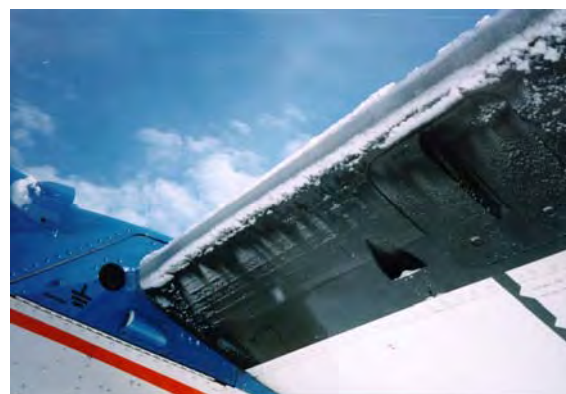
Figure 4: wind shield and wing icing after a flight of the DLR Dornier 228 aircraft in severe icing conditions.
