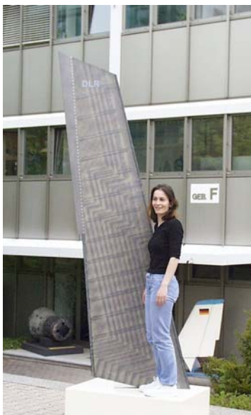
Fig 1. Experimental CFRP wing structure – demonstrator scale
