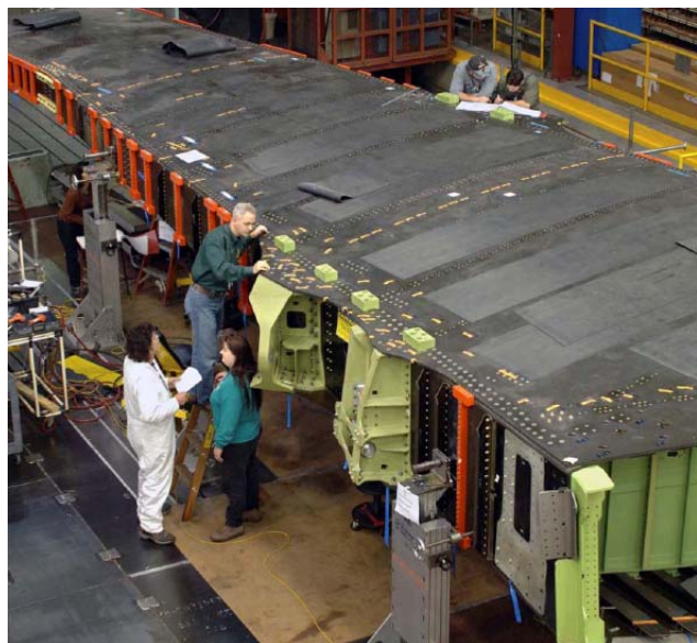
Fig. 2. CFRP wing structure of Boeing's Dreamliner – production line scale (Boeing)
