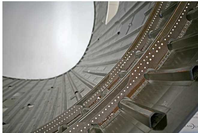
Fig. 1. Detail view of a CFRP fuselage section of Boeing's Dreamliner (Christopher Boffoli)
