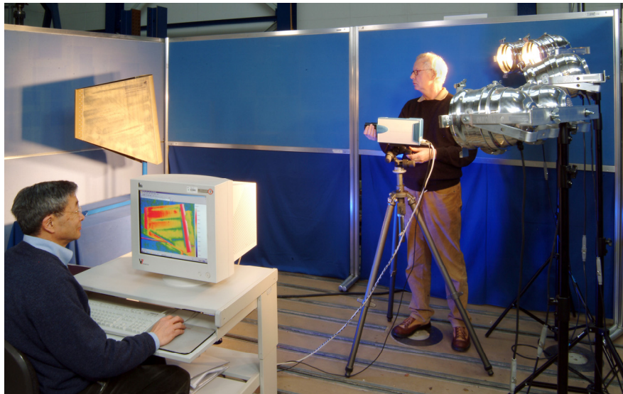
Fig. 3. Lock-in thermography analysis of a section of an aircraft rudder flap
