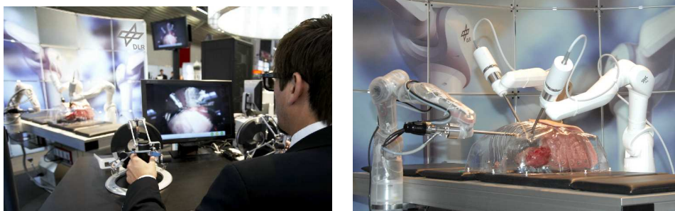
Fig. 1.1: DLR surgery scenario. Left: remote surgeon with force feedback input devices and 3D display. Right: DLR slave system consisting of three MIRO robot arms; one carrying the endoscope (semitransparent), two more carrying MIRS instruments for two handed manipulation (photos: DLR).
