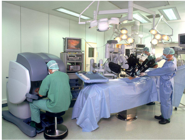
Fig. 2.3: DaVinci Surgical System from Intuitive Surgical, Inc. In the front left the master console of the system; in the center the slave-robot (photo courtesy of Intuitive Surgical, Inc., 2009).
