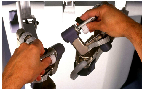
Fig. 2.5: Reestablishment of hand eye coordination in the daVinci Surgical System (photo courtesy of Intuitive Surgical, Inc., 2009).
