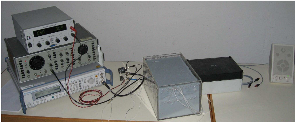
Fig. 4.1: Test-bed setup. Left top: power supply. Left middle: frequency synthesizer for the arterial pulsatile flow. Left bottom: frequency synthesizer for ultrasound transducer. Middle: acrylic glass basin filled with tissue simulating material (grey); at the front side the flexible tubes simulating the arteries running closely under the surface can be seen. In the black housing next to the basin the control electronics, the pump, and the flowmeter are situated. With the loudspeaker to the right the Doppler sounds can be made audible.
