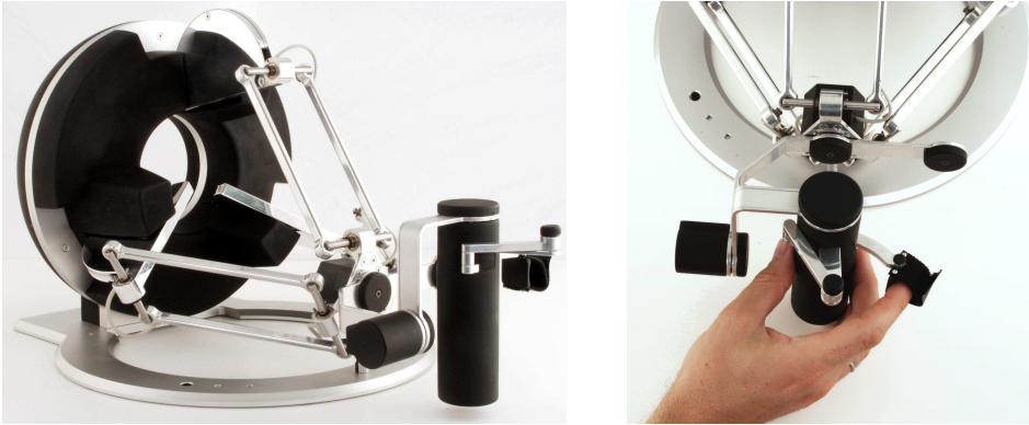
Fig. 1.2: Omega.7 seven DoF input device with 4DoF feedback (photo courtesy of Force Dimension, Inc., 2009).
