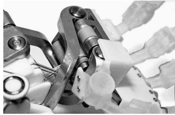
Fig. 12. Wrist integrated in forearm mockup.
