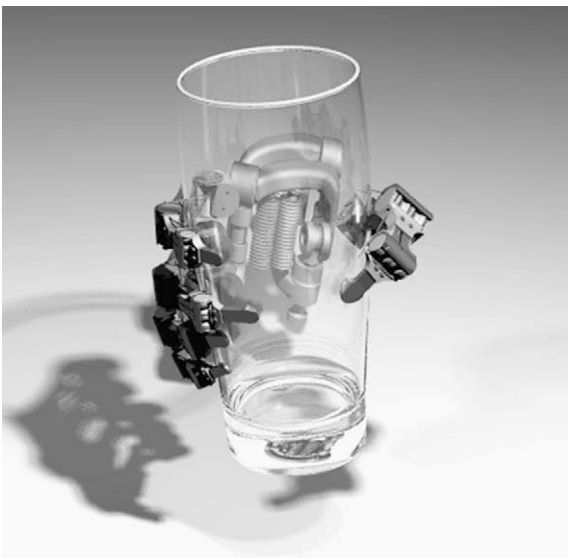
Fig. 11. Final hand design virtually grasping a 0.51 glass.
