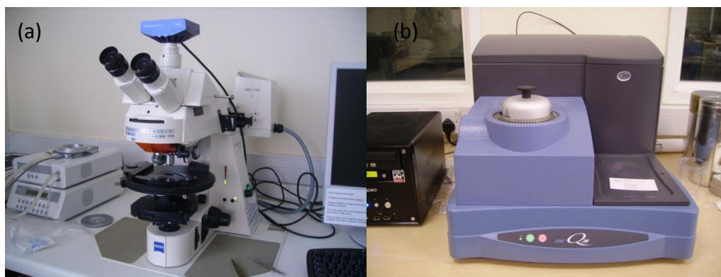
Figure 2.3. (a) A Zeiss AxioPlan2 digital microscope, and (b) Thermal analysis under a DSC Q2000 system.
