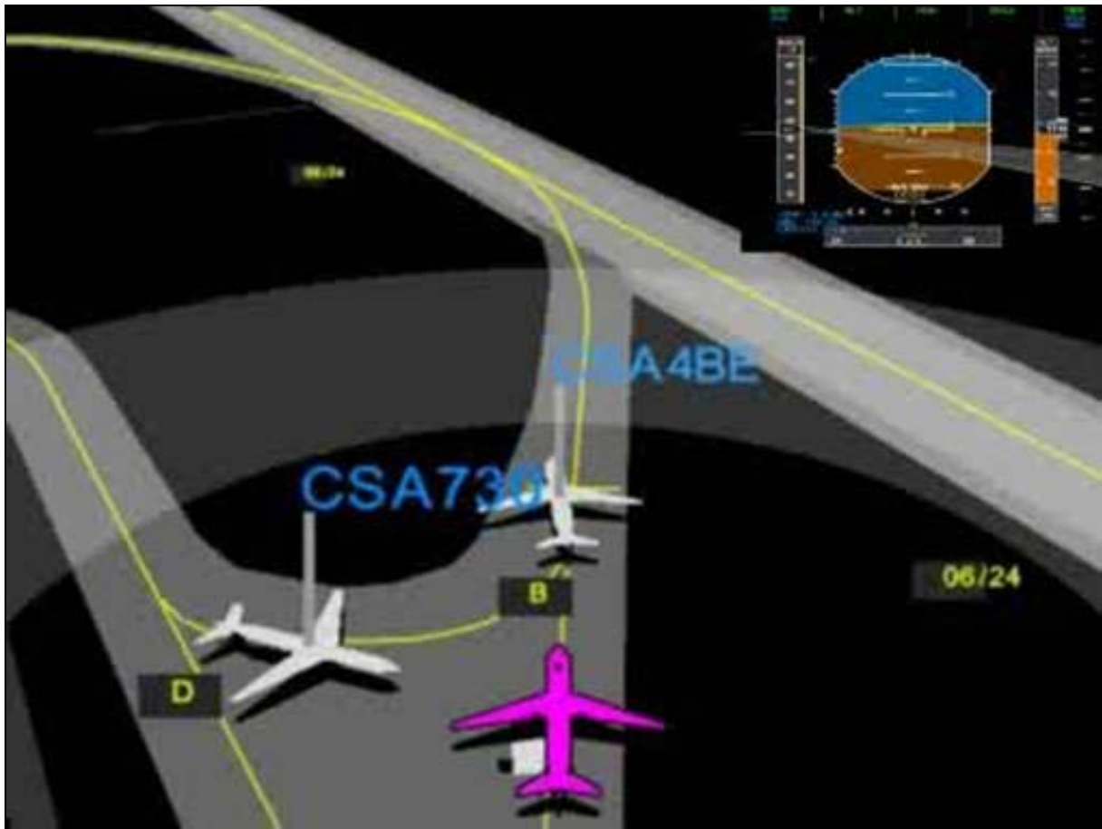
Figure 4-2: ATTAS EMM Showing Own Position (Magenta) and Surrounding Traffic
