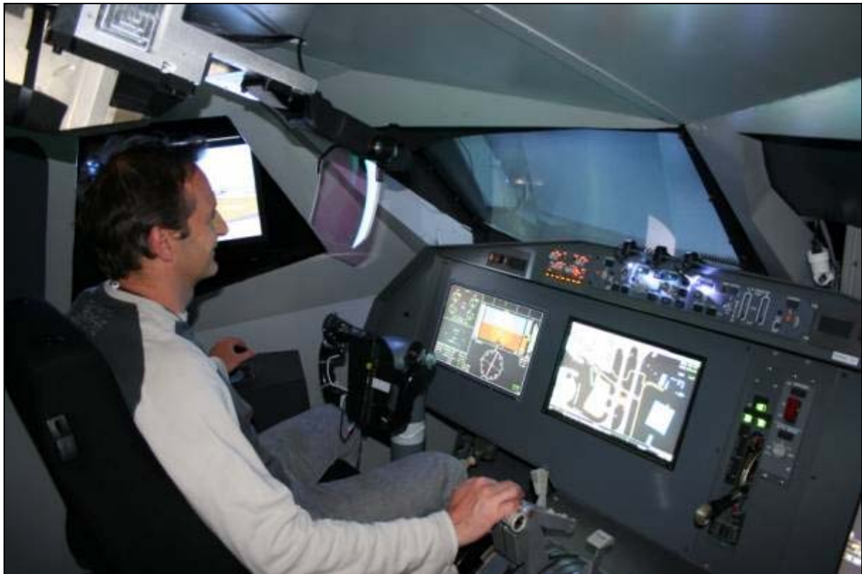
Figure 4-1: THALES Cockpit Simulator with IMM Display and HUD
