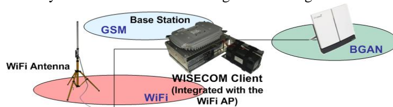
Figure 3: GSM and WiFi over BGAN architecture
