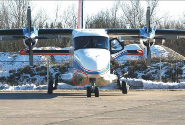
Figure 11: Photograph of the ARGOS-terminal mounted underneath the Do-228 research-aircraft (left) and terminal prior to integration (right).
