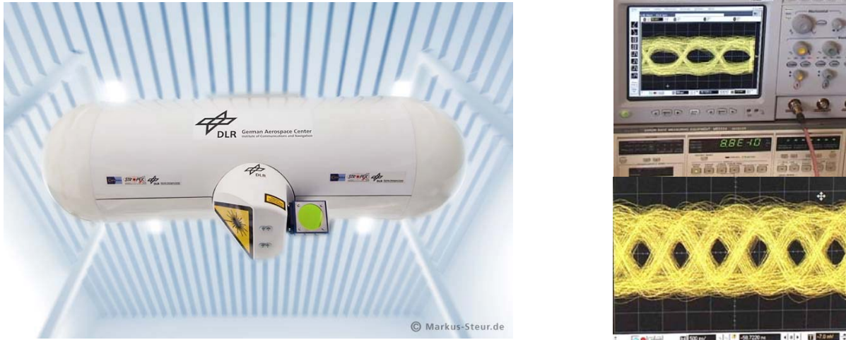
Figure 10: The CAPANINA stratospheric terminal wingpod (left) and the received data eye patterns at the ground station (right). The upper picture shows a data rate of 622 Mbit/s, the lower picture shows 1.25 Mbit/s
