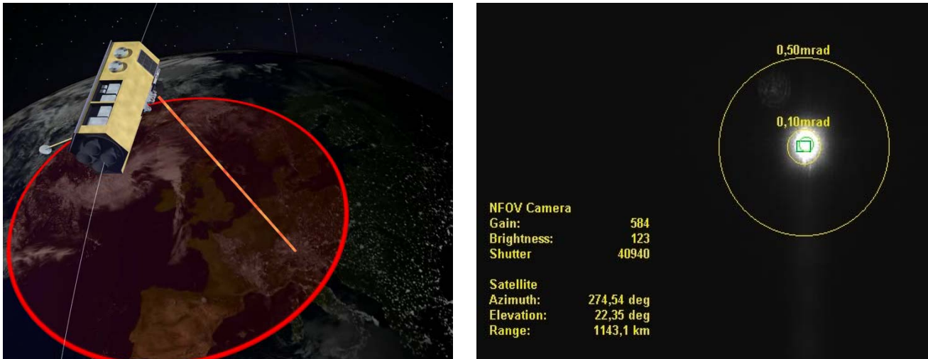
Figure 8: Scenario of LCTS-X-Downlink from TerraSAR-X (left), received signal on tracking camera of OGS-OP (right)
